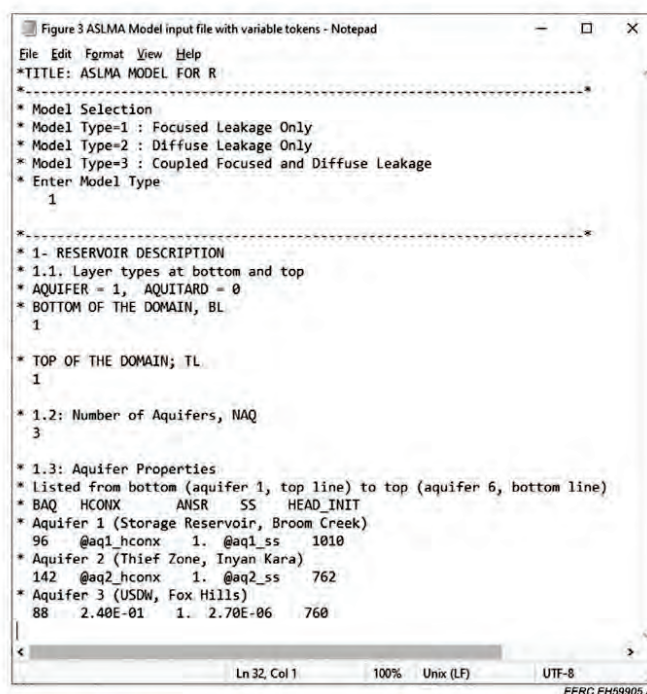
Figure 3. Example portion of ASLMA Model input file with variable tokens.
